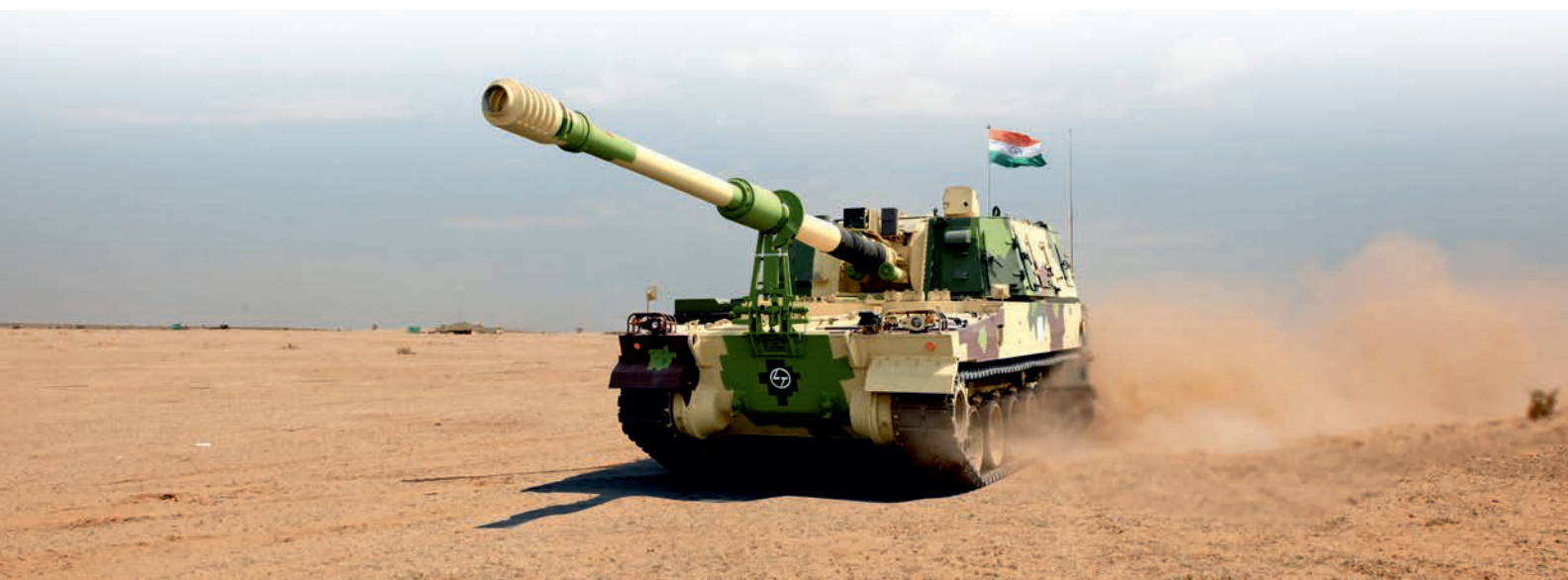
K9 Vajra-T, 155 mm, 52-calibre tracked self-propelled artillery platform, codeveloped by L&T and Hanwha Aerospace
