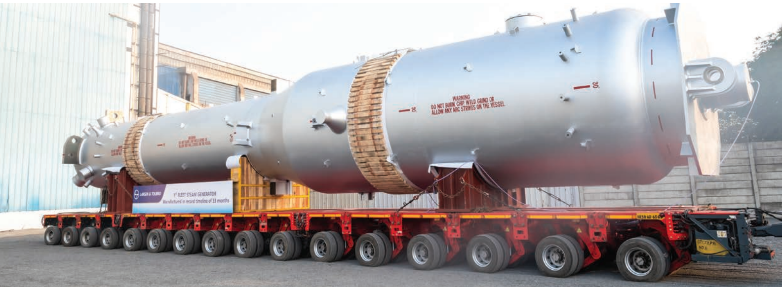
Steam Generator (SG) for Indigenously developed 10 X 700 MWe Pressurised Heavy Water Reactor, NPCIL
